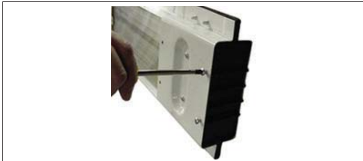
Figure 14: Tightening the Plastite® Thread-Rolling End Screws
